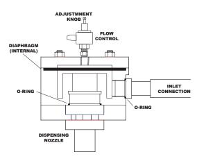
When a fill cycle is initiated, the solenoid is actuated to release air pressure on the diaphragm. At the completion of the fill, the solenoid is actuated again to restore pressure on the diaphragm -sealing the flow of product through the outlet connection.
